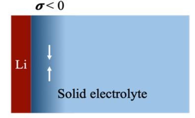
**Compressive** surface stress prevents Li dendrite penetration
